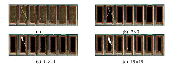
Figure 8. Effect of neighborhood window sizes for the gold fingers with a nick: (a) The original image. (b)-(d) The processing results from window sizes 7×7, 11×11 and 19×19, respectively.
